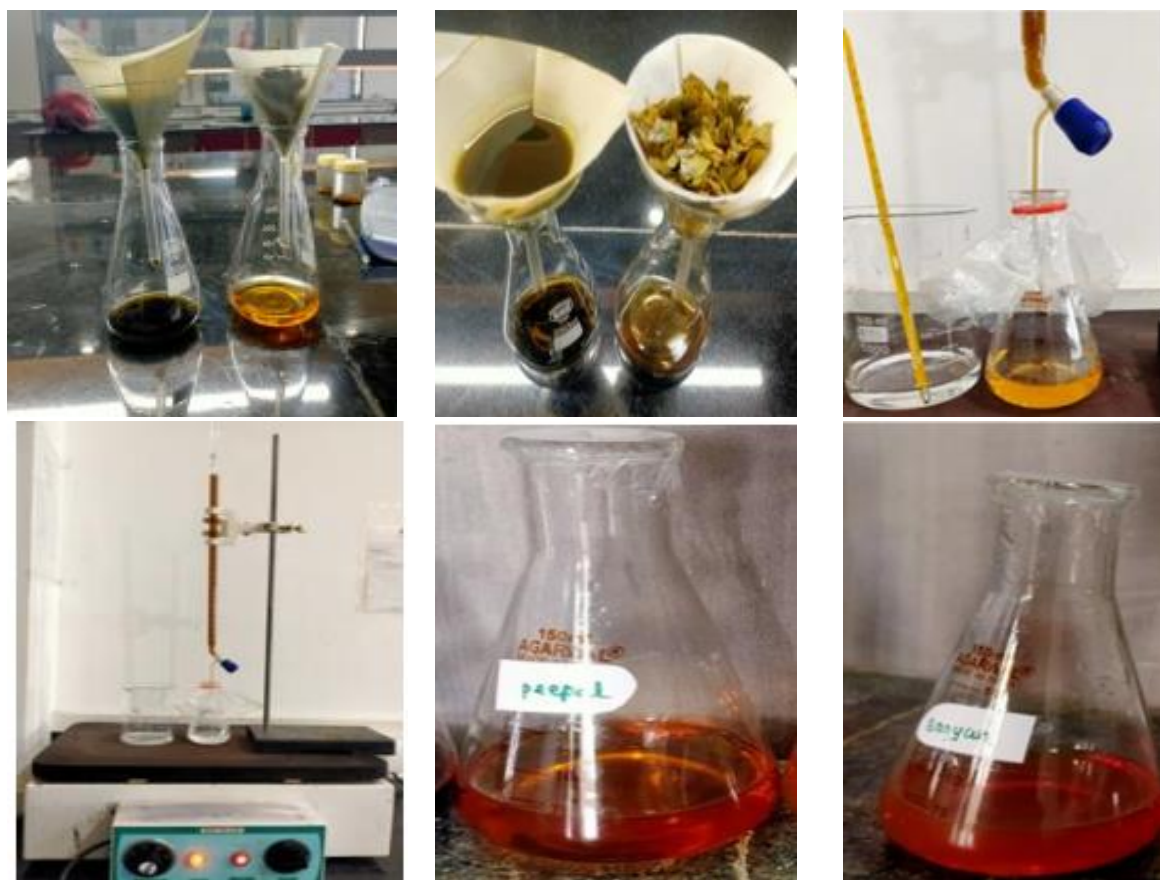
Fig 1 Biosynthesis of silver nanoparticles from leaf extract
