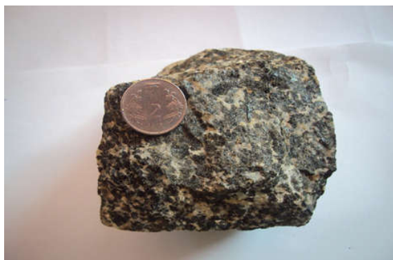
Figure 9: Hybrid rock with pyroxene cumulates
