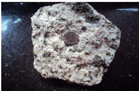
Figure 8: Hand specimen of syenite with pyroxene clots
