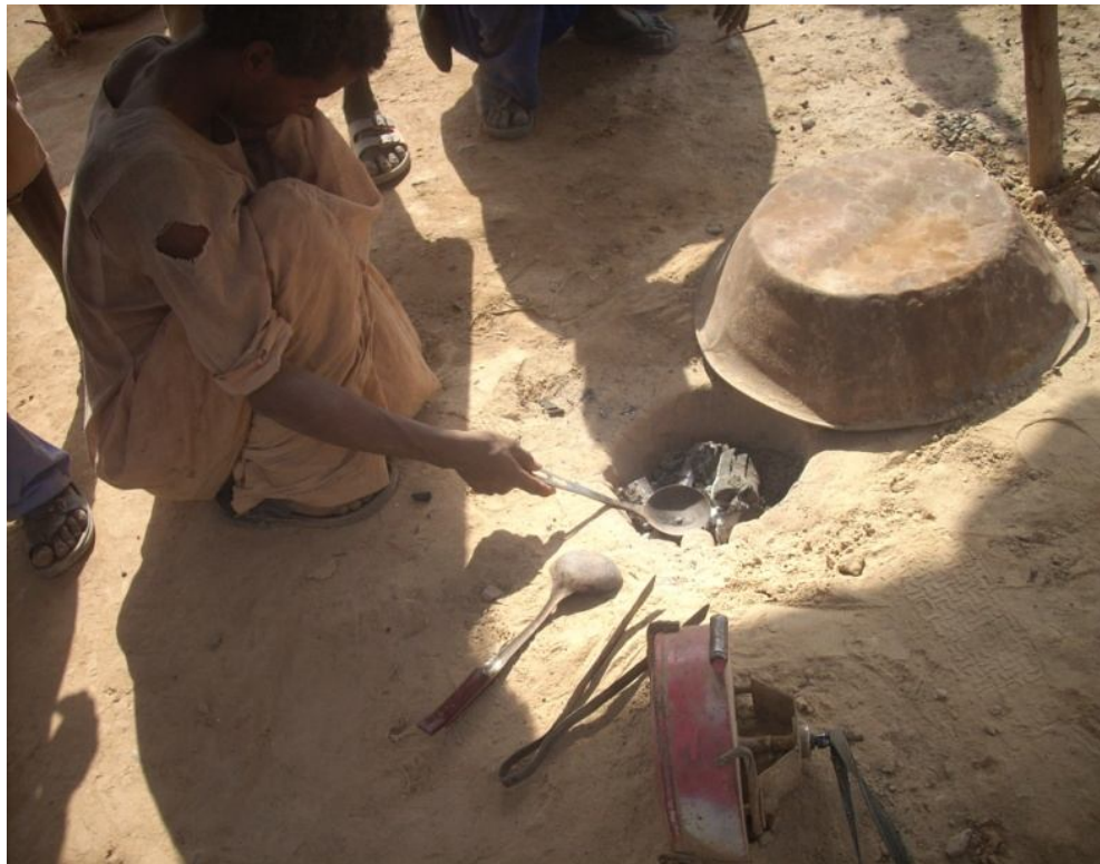
Fig. 7: The mercury evaporates and the gold is left
