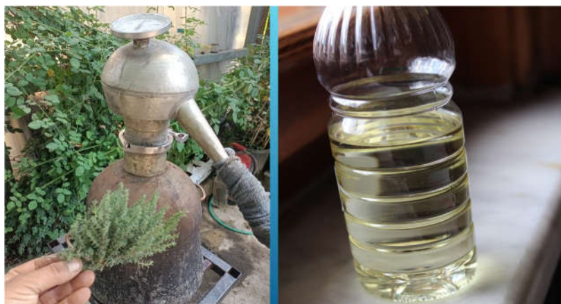
Figure 5: Production of rosehip oily water (hydrosol) by imbik (local production aparat).
